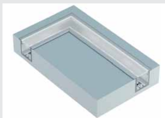
Example of installation 90° corner (45° cut to be done)
