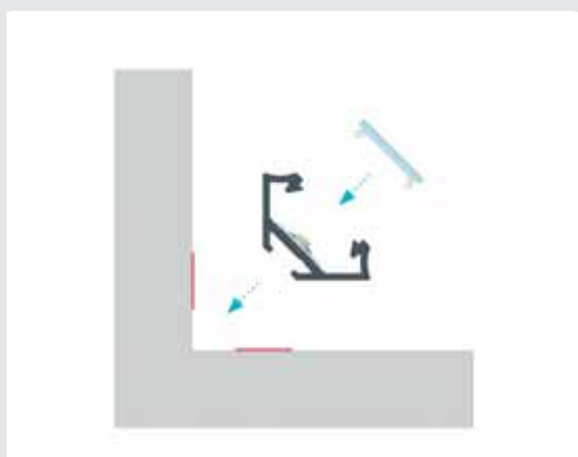
Fixation with a bi-adhesive tape plus cover clicking
