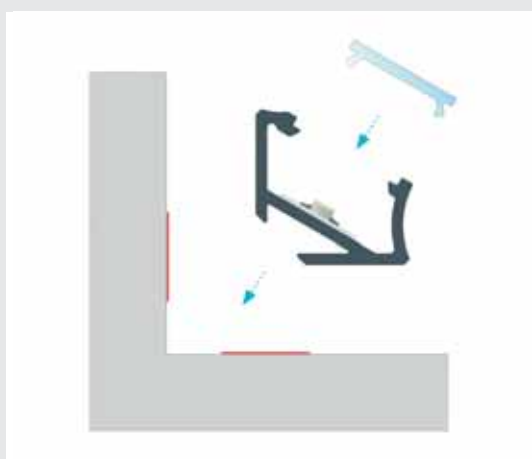
Fixation with a bi-adhesive tape plus cover clicking
